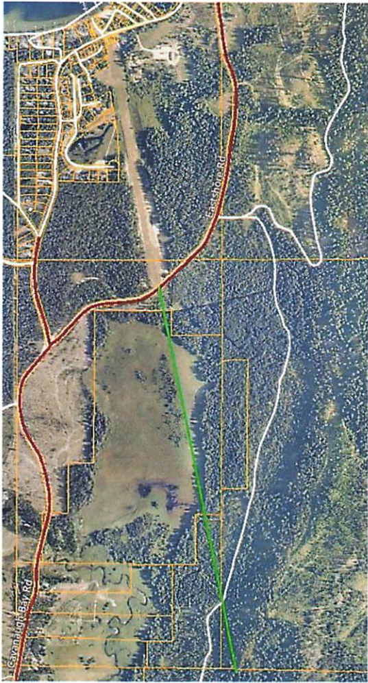
Figure 3 Cavannaugh Bay airstrip showing 5000 feet of critical area into private properties
